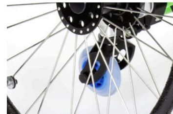
Telescoping, removable anti-tipper provides safety for novice racers.
