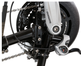
Cable driven shifting for upper chain rings.
