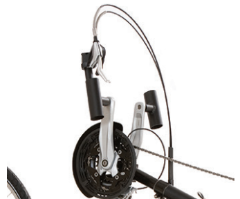
Shimano® components for hands-on shifting and braking.
