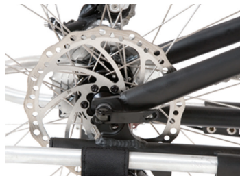
Front disk brake and welded footrest clamps.
