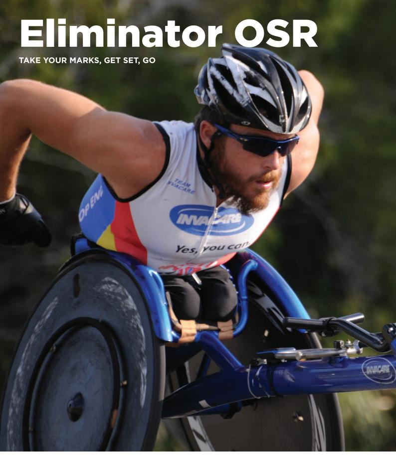
The Top End® Eliminator™ OSR is designed for speed! This comes thanks to its super-stiff formed horizontal main tube, combined with a relaxed headtube angle for stability and aerodynamics. It offers a range of different cage designs custom built to accommodate a multitude of abilities and positions.
