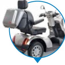
Improved, secure lockable rear storage Front storage for items such as glasses and mobile phone
