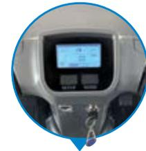
Bright, easy to read LCD display control panel indicates speed, driving length, working hours' counter, battery status, lighting and signing.
